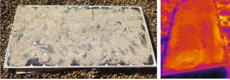
**Fig. 9.** Solar panels totally covered of dirt
