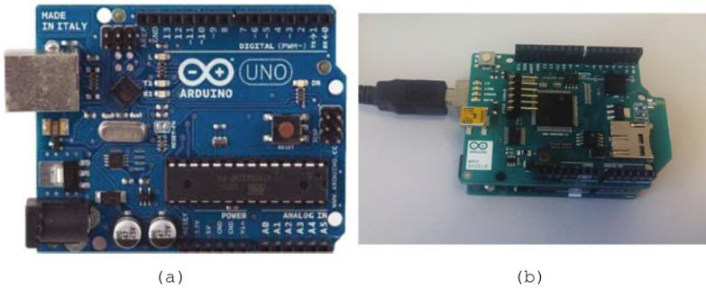
Fig. 3. Arduino Uno G3 (a) and Wi-Fi Shield expansion card (b)
