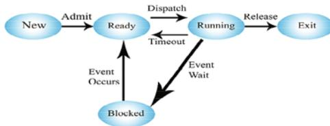
Fig. 2. Five state model for process states
