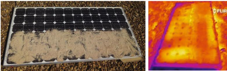
**Fig. 8.** Solar panels covered in half of mud
